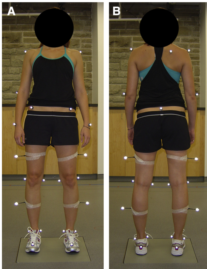
Fig 2 Anterior (A) and posterior (B) views of the modified Helen Hayes marker set used for 3-dimensional gait analysis.
